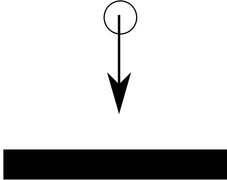
The material properties for both the particle and wall are: Young's modulus is  $80 \cdot 10^9 \text{ Pa}$ , Poisson coefficient is 0.20, and the particle material density is  $3000 \text{ kg/m}^3$ .
