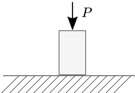
b) Next, we replace the punch with a single force (also 10000 N). Calculate the surface deformation at a distance of  $r = 2$  cm from the force location
